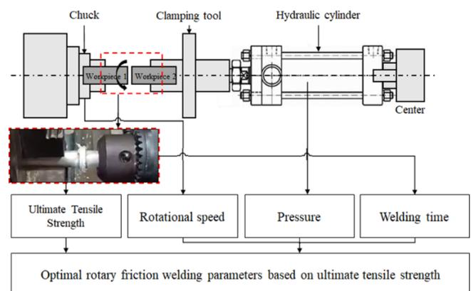
**Figure 1.** Schematic diagram of experimental setup of the rotary friction welding operation.
