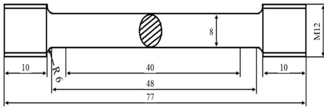
Figure 2. Specimen of the tensile test according to DIN 50125 type B.
