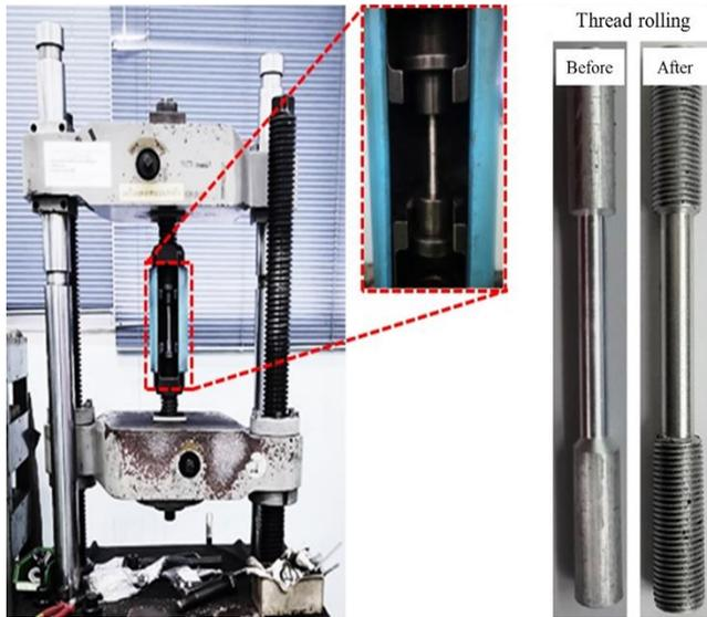
Figure 3. Universal testing machines and rotary friction welding specimen before thread rolling and after thread rolling.
