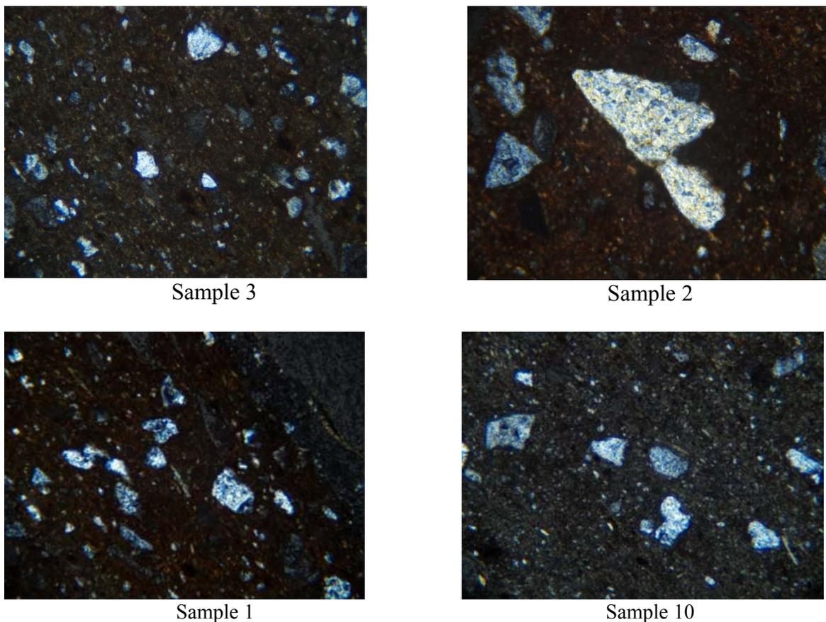
**Figure 4.** Single-quartz grains in soil texture
