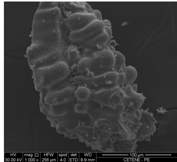
Figure 4. Morphology of showing nodules islands of quasicrystalline alloy Al_{62,2}Cu_{25,3}Fe_{12,5} ,
