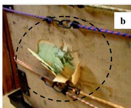
**Figure 3** Testing of aramid fabric with .357 magnum: (a) penetration of the bullet at the front of the modeling clay and (b) the thrown off at the back of the modeling clay box.
