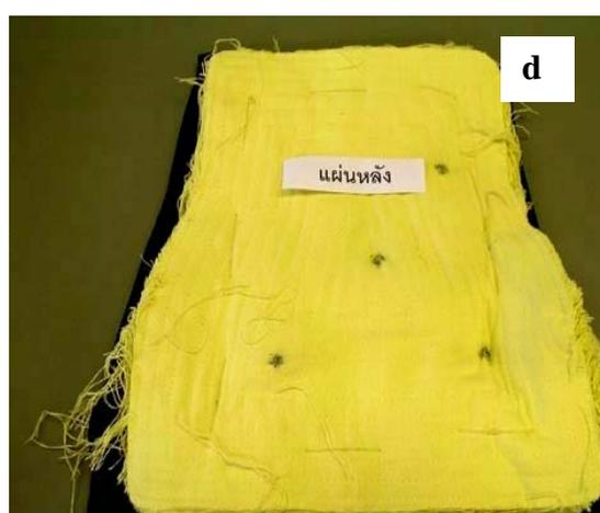
**Figure 6** Testing of bulletproof vest from bullet impact: (a) clamping the vest with modeling clay; (b) indentation of modeling clay after the bullet impact on the vest (front size); (c) bullet blocked in the front size of the vest and (d) bullet blocked in the back size of the vest.
