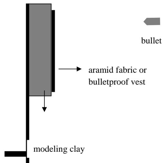
**Figure 1** Schematic diagram of the ballistic test.
