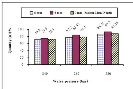
**Figure 9.** Yield quantity (%wt) of Copper powder obtained from 10 kg of raw metal.
