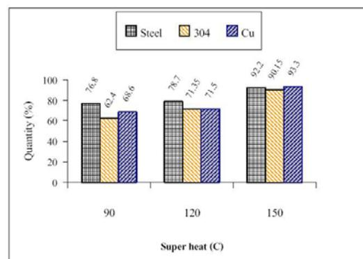
**Figure 11.** Powder Yield Quantity from  $\varnothing$ 6 mm Nozzle.
