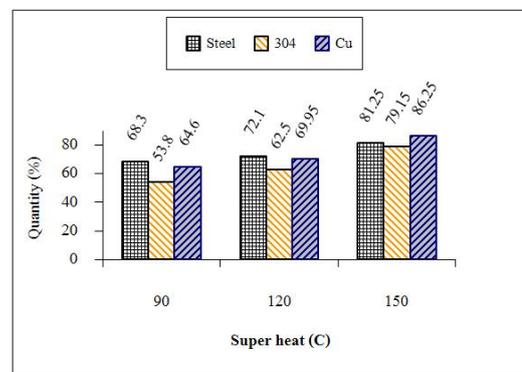
**Figure 10.** Powder Yield Quantity from  $\varnothing$ 5 mm Nozzle.
