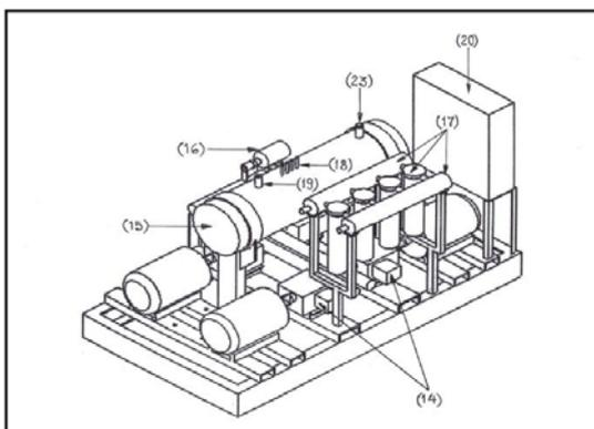
**Figure 2.** Full Set of High Water Pressured Pump with 280 bar and Flow Rate at 80 liters/min.
