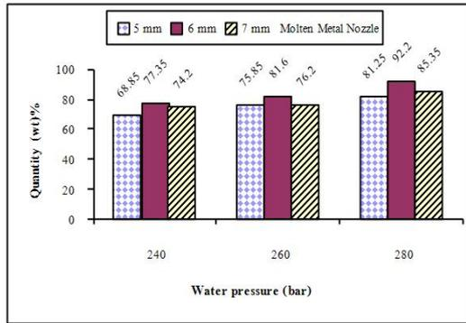
**Figure 7.** Yield quantity (%wt) of low carbon steel powder obtained from 10 kg of raw metal.
