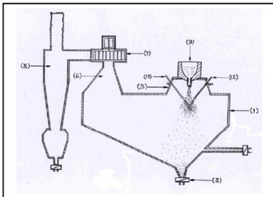
**Figure 1.** Internal Description of a Water Atomizing Machine.
