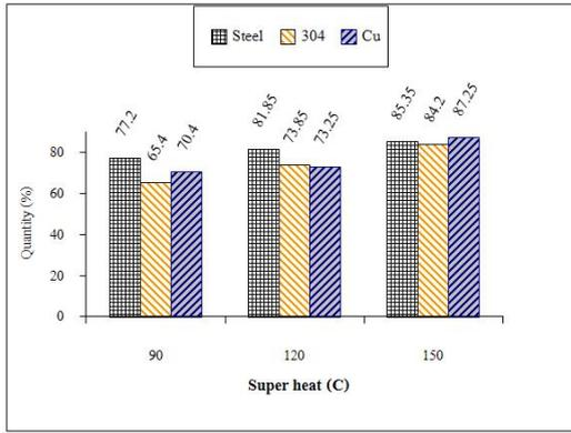
Figure 12. Powder Yield Quantity from Ø7 mm Nozzle.
