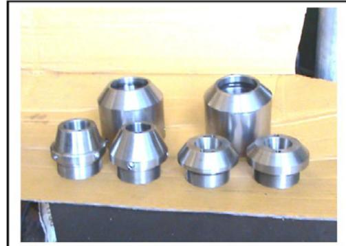
**Figure 5.** Changeable Cone Nozzles.
