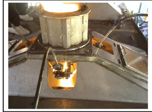
**Figure 3.** Molten Metal Spraying by V-jet Nozzle.
