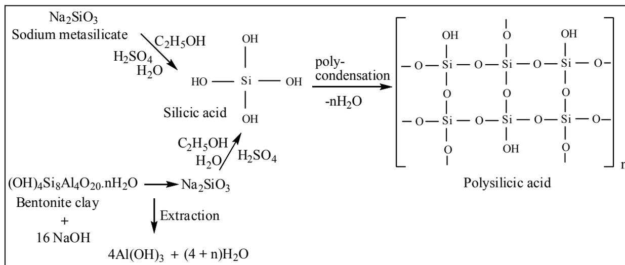
**Figure 2.** Hydrolysis and polycondensation of sodium metasilicate and bentonite clay.
