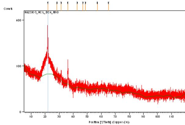
Figure 6a. XRD patterns of the SMS based monolith.
