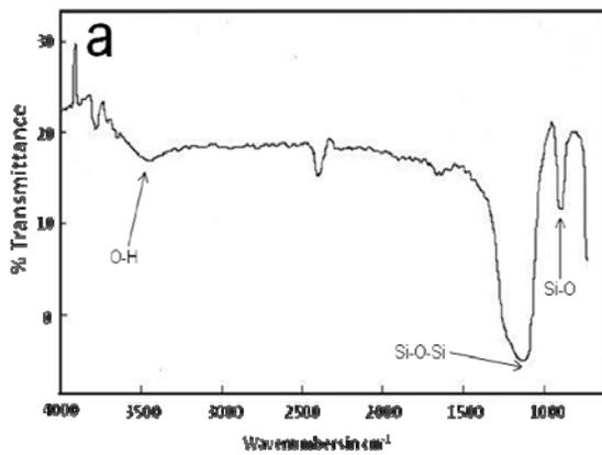
Figure 5a. FTIR spectra of SMS monolith.
