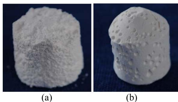
**Figure 4.** Monolith from (a) sodium metasilicate, and (b) bentonite clay.
