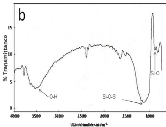
Figure 5b. FTIR spectra of BTC monolith.
