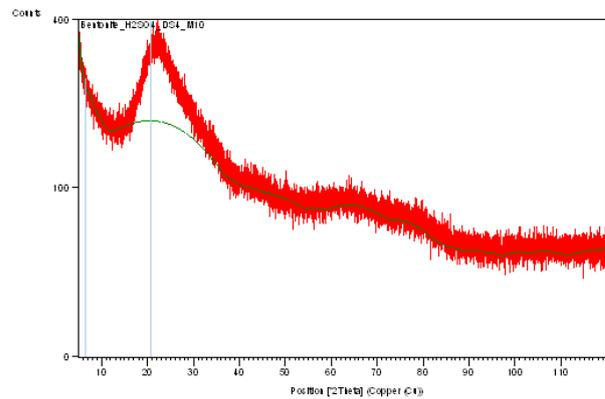
Figure 6b. XRD patterns of the BTC-based monolith.
