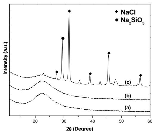
**Figure 2.** X-ray diffraction patterns for (a) Washed pure silica gel and (b) Blue silica gel impregnated with  $\text{CoCl}_2 \cdot 6\text{H}_2\text{O}$  ( $2.1 \times 10^{-3} \text{ mol} \cdot \text{dm}^{-3}$ ) and (c) Unwashed Silica gel.
