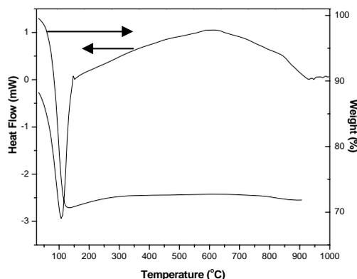
**Figure 6.** DSC/TG of Humidified Blue Silica Gel
