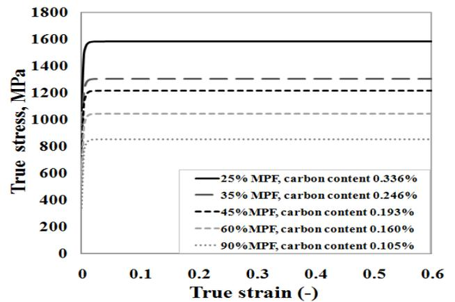
**Figure 7:** Modeled flow curves of martensite in the investigated DP steels having different MPF values and carbon content.
