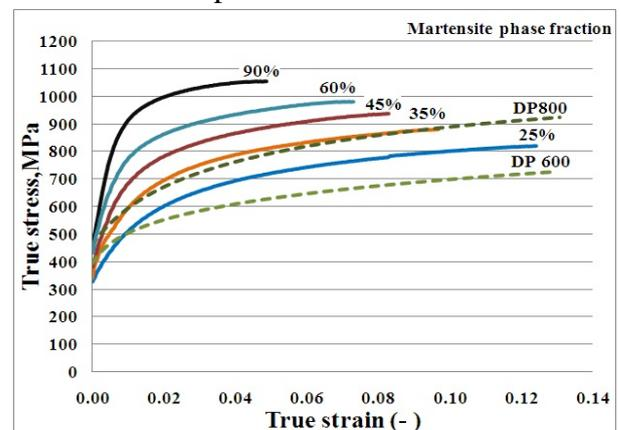
**Figure 2.** Results of tensile tests for different annealed DP steels in comparison with commercial DP600 and DP800 steel.
