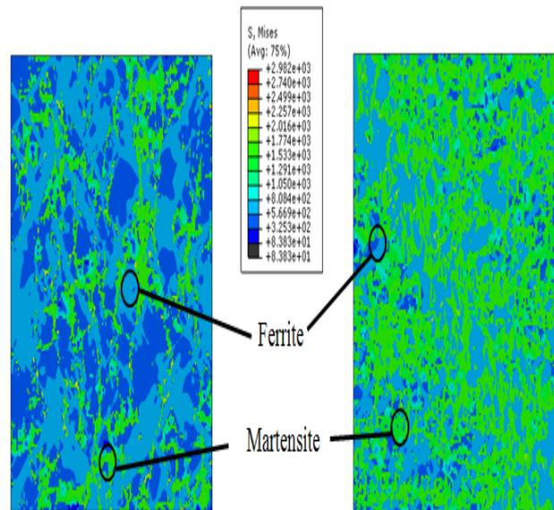
**Figure 9:** Local stress distribution in the DP microstructure with (a) MPF of 25% (b) MPF of 60% at uniaxial tensile strain of 10%.
