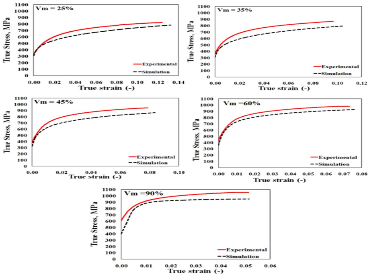
**Figure 8:** Comparisons between experimental and numerical flow curves of the investigated DP steels with varying martensite contents.
