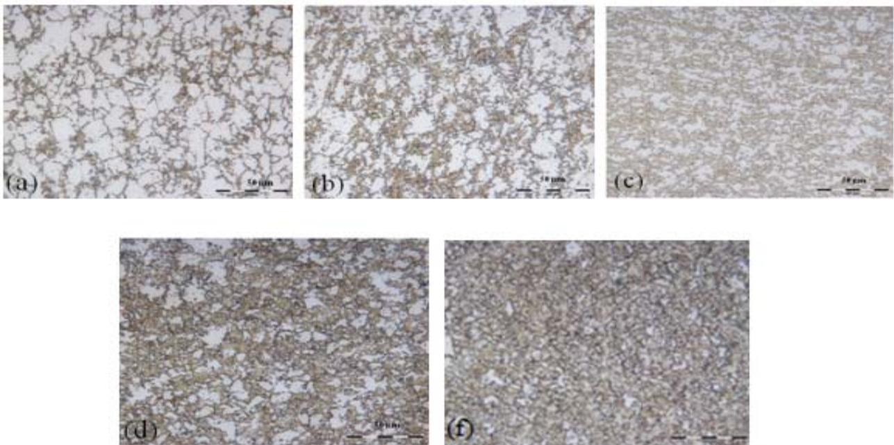
**Figure 3 :** Optical micrographs of the investigated DP steels with the MPF of (a) 25%, (b) 35%, (c) 45%, (d) 60%, and (f) 90%.
