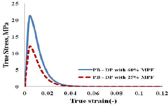
**Figure 5 :** Stress - strain curves representing phase boundary hardening for DP steels with 25% and 60% martensite.
