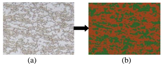
**Figure 4:** (a) Micrograph of the investigated DP microstructure with MPF of 45% and (b) corresponding generated 2D RVE model with 130x170 elements.
