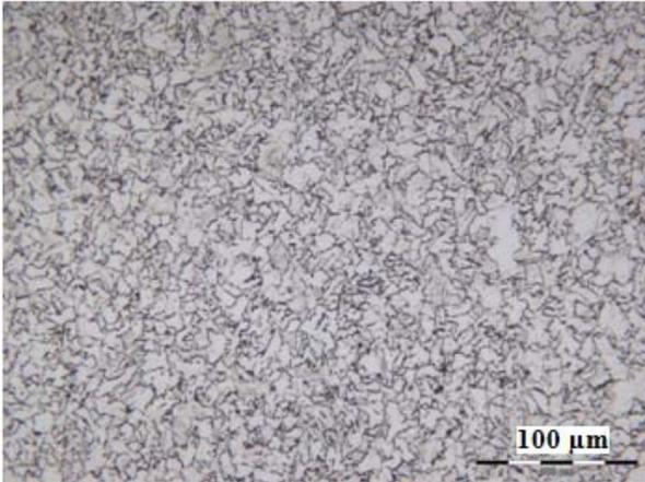
**Figure 1 :** Microstructure of the as-received steel sheet.
