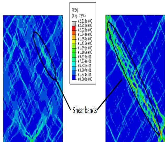
**Figure 10:** Local strain distribution in the DP microstructure with (a) MPF of 25% (b) MPF of 60% at uniaxial tensile strain of 10%.
