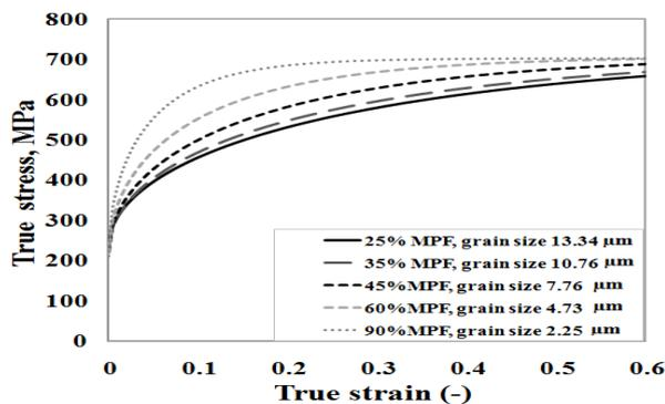
**Figure 6 :** Modeled flow curves of ferrite in the investigated DP steels having different MPF values and ferritic grain sizes.
