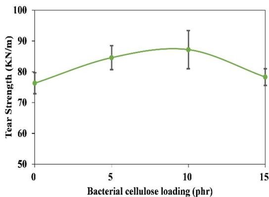
Figure 7. Tear strength of NRL filled with BC composites.
