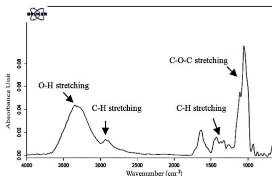
**Figure 1.** FTIR spectra of bacterial cellulose (BC).
