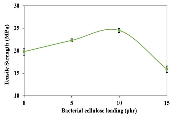
**Figure 4.** Tensile strength of NRL filled with BC composites.
