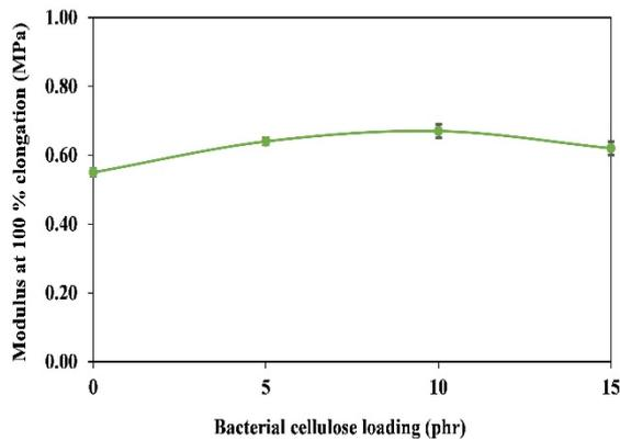
Figure 6. Modulus at 100% elongation (M100) of NRL filled with BC composites.
