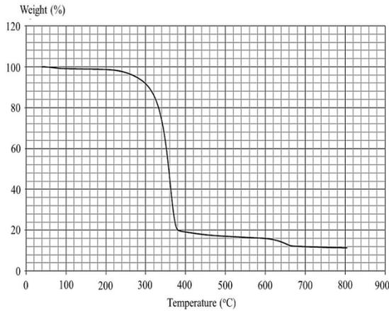
**Figure 2.** TGA thermogram of BC.
