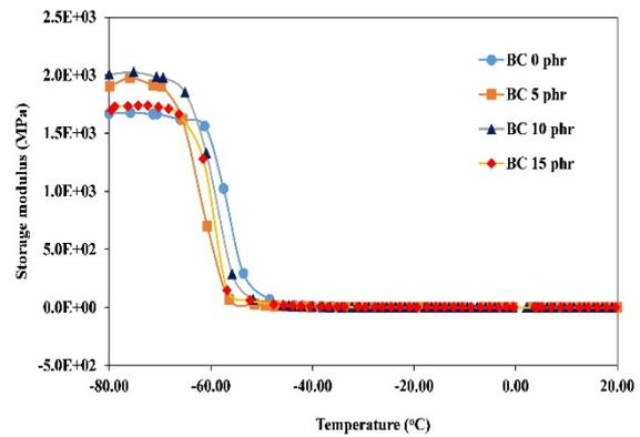
Figure 8. Storage modulus of NRL filled with BC composites.
