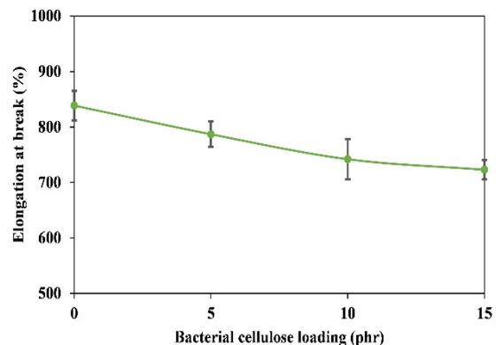
**Figure 5** Elongation at break of NRL filled with BC composites.
