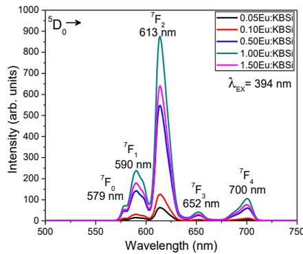
**Figure 5.** Emission spectra of KBSi:Eu<sup>3+</sup> glasses in the range of 500 to 750 nm.
