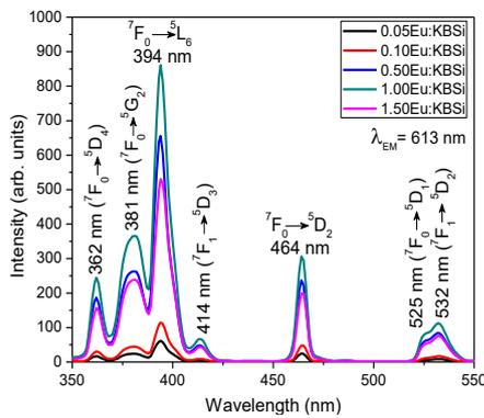
**Figure 4.** Excitation spectra of KBSi:Eu<sup>3+</sup> glasses in the range of 350 to 550 nm.
