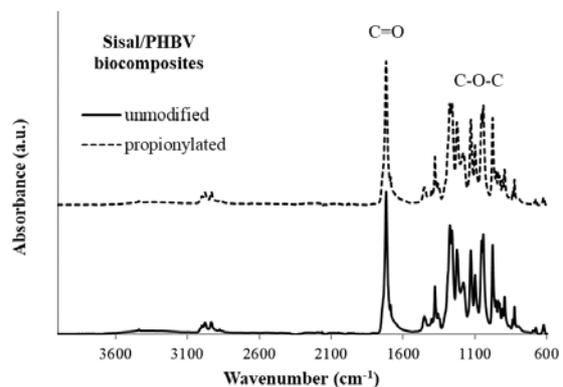
**Figure 1.** FTIR spectra of sisal fibre/PHBV biocomposites.
