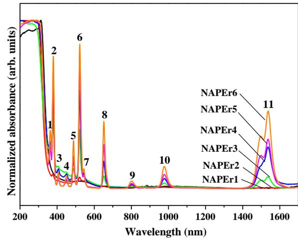
Figure 2. The absorption spectra of the glass samples with different Er<sub>2</sub>O<sub>3</sub> concentration.
