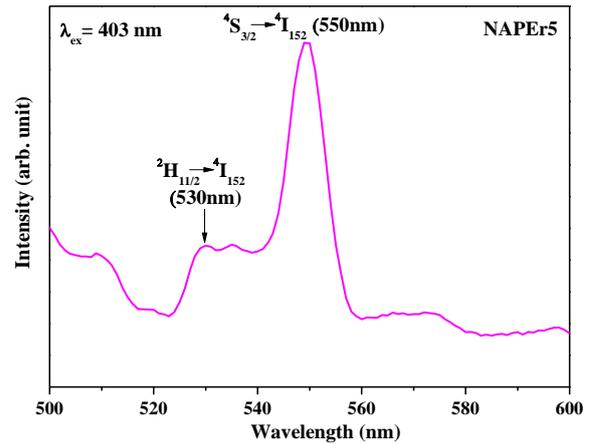
**Figure 5.** Visible emission spectra of NAPER5 glass under the excitation of 403 nm.
