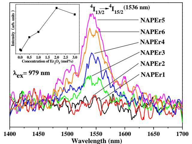
**Figure 3.** NIR photoluminescence spectra from  $^4I_{13/2} \rightarrow ^4I_{15/2}$  transition of NAPER glasses.
