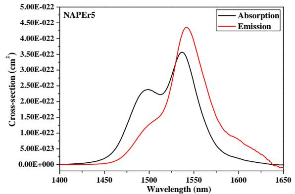
**Figure 6.** Absorption and emission cross-sections for <sup>4</sup>I<sub>13/2</sub>→<sup>4</sup>I<sub>15/2</sub> of Er<sup>3+</sup> doped NAPER5 glass calculated by the McCumber theory.
