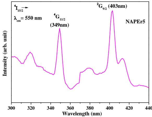
**Figure 4.** Excitation spectra of NAPER5 glass under the emission of 550 nm.
