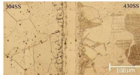
**Figure 3.** The microstructure of the joint zone at a temperature of 1120°C and 60 min.
