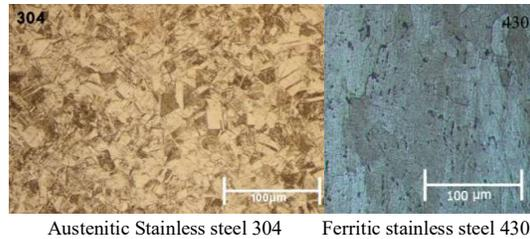
**Figure 1.** Crystal structure of base metals before the joint.
