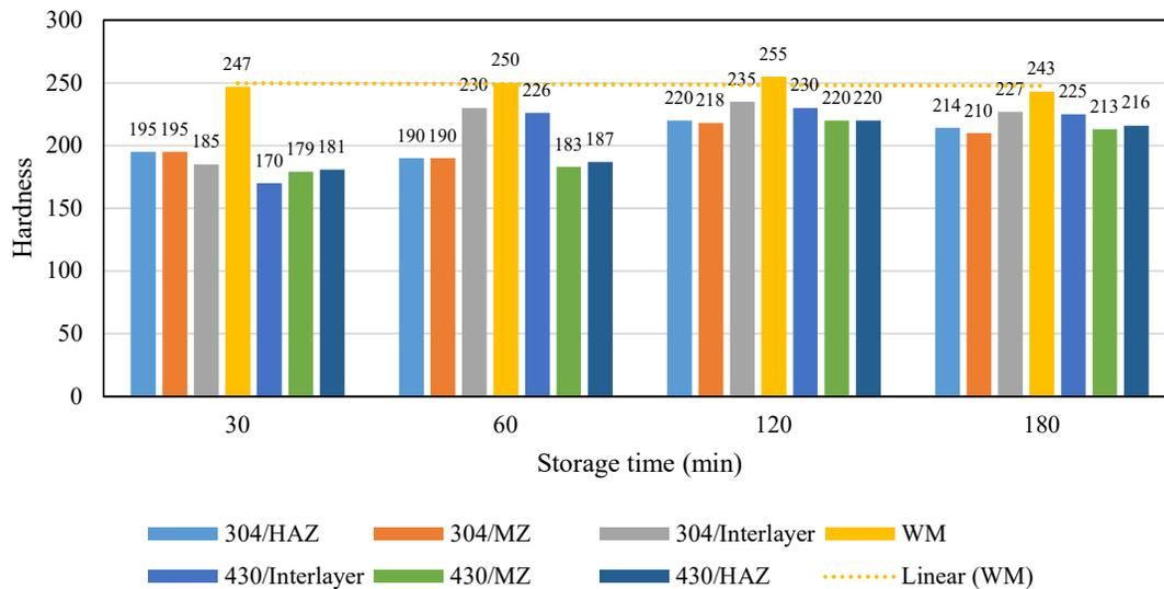
Figure 9. The statistical chart of hardness values of junction.
