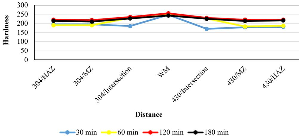
Figure 8. Hardness of different dough areas, mashi zone, heat affected zone, seamless joint at a temperature of 1120°C and storage time of 30, 60, 120, and 180 min.
