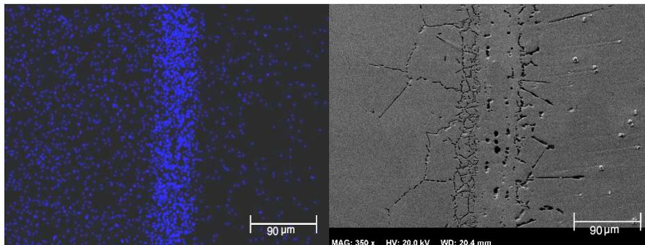
**Figure 6.** The amount of nickel element dispersion in the joint: (a) The amount of nickel element dispersion in base metals, (b) The SEM image of joint.
