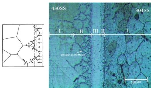
**Figure 2.** The microstructure of the joint zone at 1120°C and 30 min.
