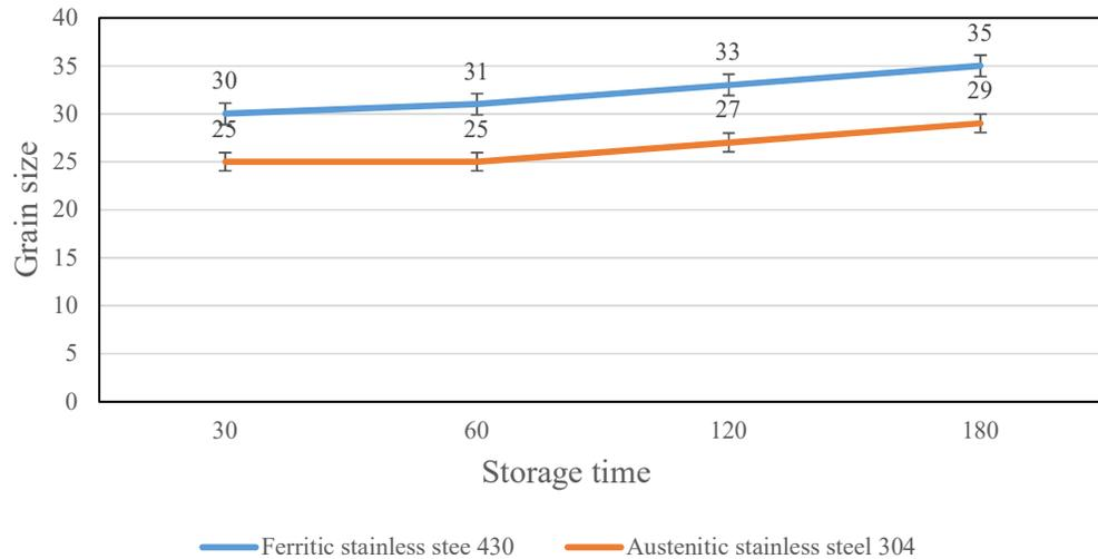
**Figure 7.** Density changes in grain relative to the storage time of 30, 60, 120, and 180 min at a constant temperature of 1120°C.
