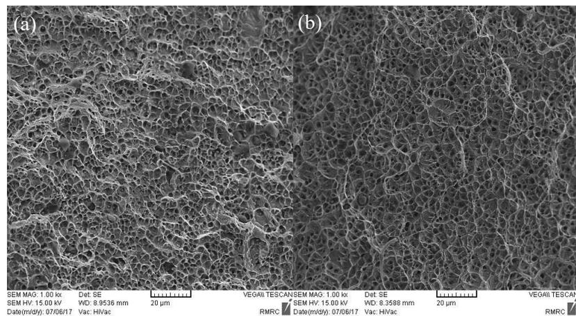
**Figure 11.** Microscopic image of the failure levels in the shear strength of the joint in (a) storage time 120 min and (b) storage time 30 min.
