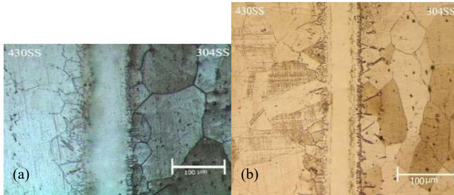
**Figure 4.** Joint microstructure (a) Temperature of 1120°C and 120 min of storage time; (b) Temperature of 1120°C and 180 min of storage time.
