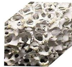
Figure 6. Picture of porous PZT, whose holes are to be filled with a polymer, forming a 3-3 connectivity.
