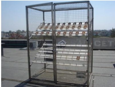
Figure 1. Atmospheric exposure racks with samples exposed in it.
