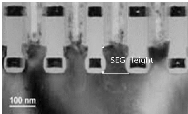
Figure 5. (a) TEM image of SEG height (b) The comparison of un-doped SEG vs. boron doped SEG height variation.
