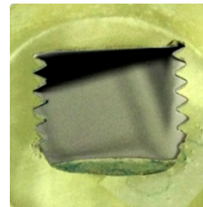
Figure 2. Cross section of a bolt from GN group as prepared for hardness measurement
