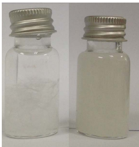
(A) (B) Figure 1. Suspensions of (A) bamboo fibers and (B) MFC fibrils after 60 minutes treatment time.
