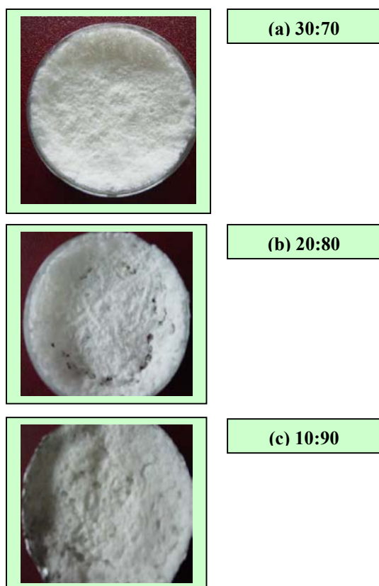
Figure 4 Photographs of foam samples with various ratios of starch-g-polystyrene and water (a) 30:70, (b) 20:80, and (c) 10:90
