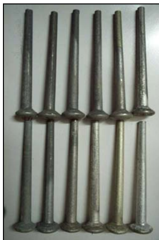
Figure 1 As cast specimens using the induction caster machine with vacuum system. Silicon content added in the specimens from left hand to right hand as follows. 0, 0.1, 0.2, 0.3, 0.4 and 0.5 % by weight (Top row : Silver grade 925 and bottom row : Silver grade 950)
