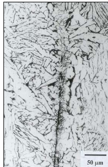
Figure 7 The microstructure of sample close to fracture surface (steel C, T = 800^\circ\text{C} ).
