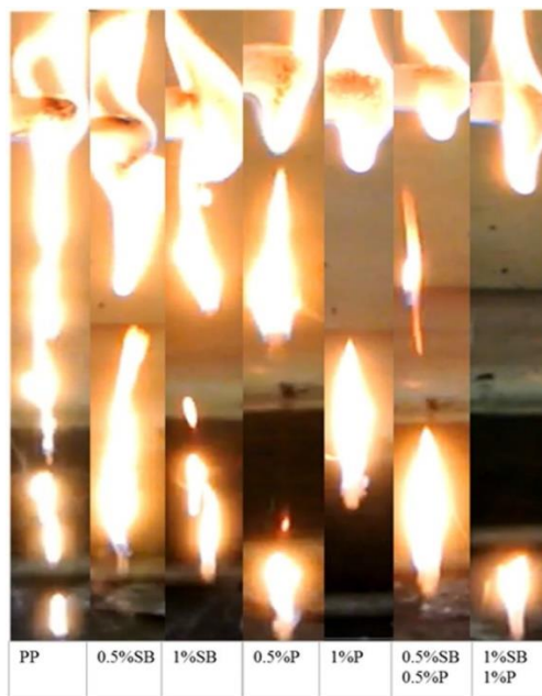
Figure 10. Horizontal burning test of binary and ternary composites containing soybean oil-g-chitosan and phosphonated silica.
