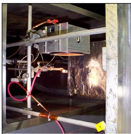
Figure 3 Image of apparatus for electrospinning of polymer melts in a vacuum as outline in figure 2. The radiant heat source is in the metal box at the top center. The nanofibers collected on the wrinkled aluminum sheet are visible on the right hand side of the figure. The spinneret is immediately below the radiant heater.
