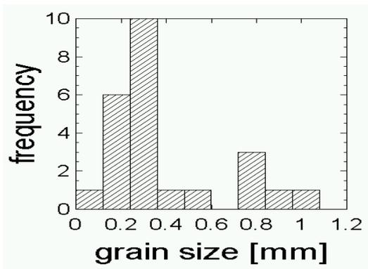
**Figure 9.** Frequency of the estimated austenite grain size
