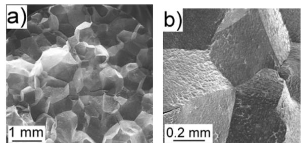
**Figure 8.** High temperature fractures, intensity of the reduction of area drop 4
