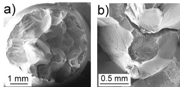
**Figure 7.** High temperature fracture, intensity of the reduction of area drop 3
