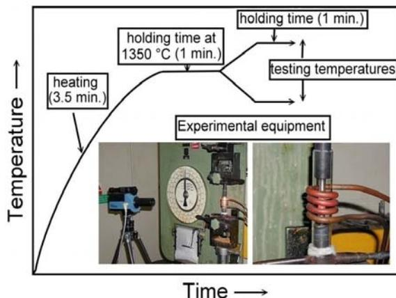
**Figure 1.** Heating up of specimens and the experimental equipment
