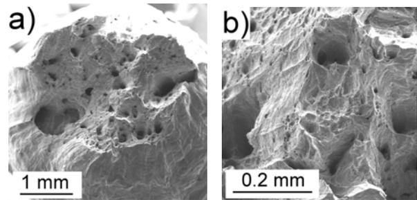
**Figure 5.** High temperature fracture, intensity of the reduction of area drop 1.5
