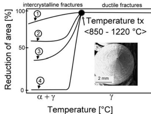
**Figure 2.** Scheme of a decrease of the reduction of area values and its classification
