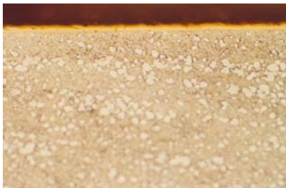
Figure 6a TiN coating of thickness 2 \mu\text{m} deposited on polished high - speed steel substrate. Magn. 1000x, etched
