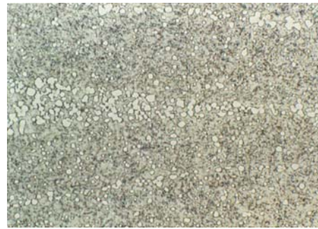
Figure 1 Microstructure of etched high – speed steel after heat treatment
