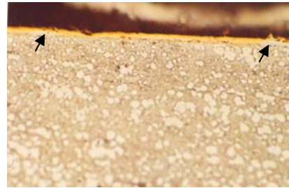
Figure 6b TiN coating of thickness 2 \mu\text{m} deposited on polished and etched high – speed steel substrate and showing some coating defects. 1000x
