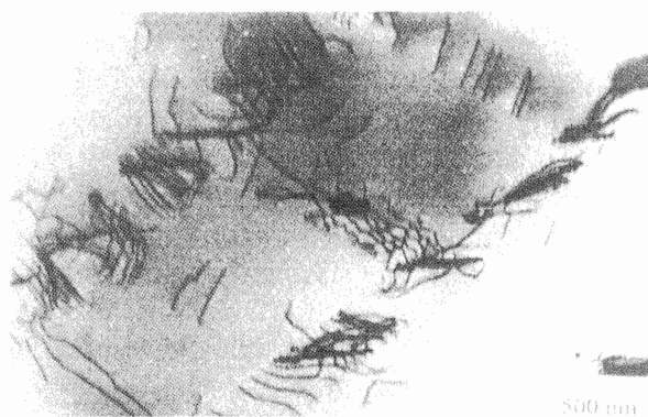
Figure 9 Dislocation pile-ups at precipitate particle after 50 minutes annealing.
