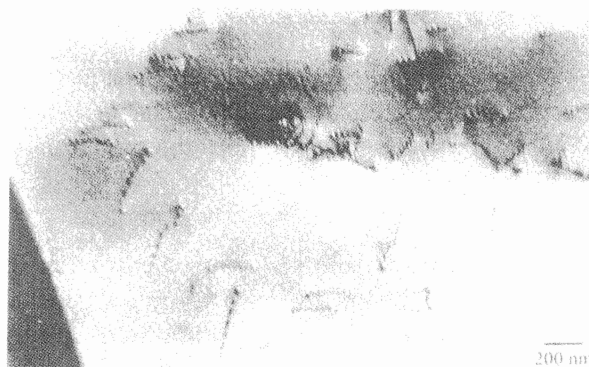
Figure 7 Lower density of dislocation structure in recrystallized grain after 10 minutes.
