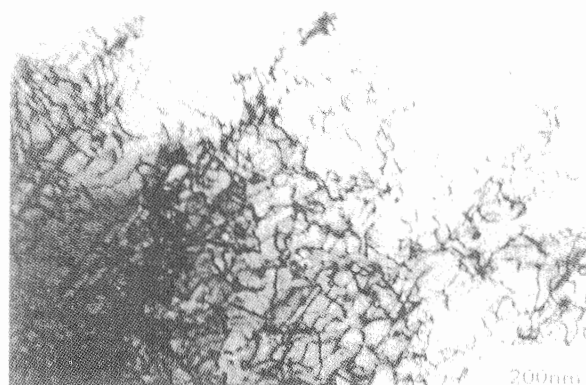
Figure 1 The very dense and homogeneous dislocation tangles in deformed grain, A1.
