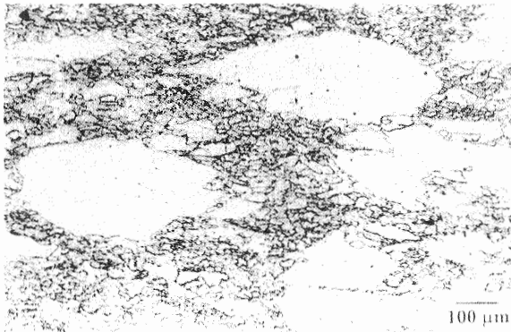
Figure 3 Micrograph of quenched microstructure, A1.
