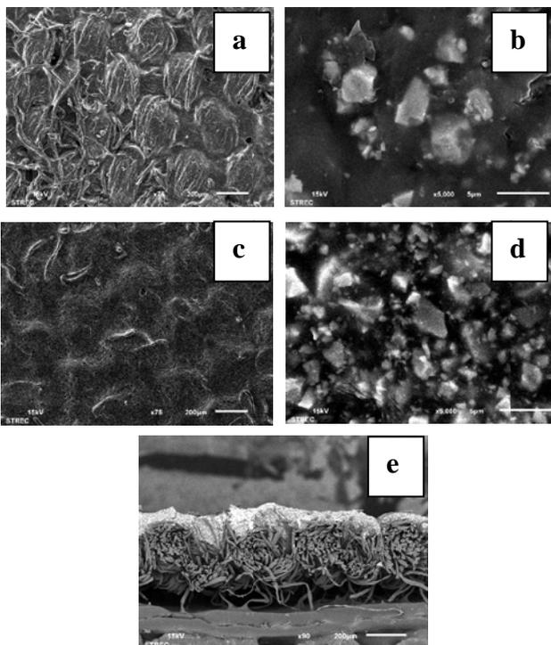
**Figure 1.** SEM micrographs of the coated fabrics with barium sulphate at different concentration: (a-b) 10% (w/w); (c-d) 50% (w/w) and (e) cross section of the fabric coated with 50% (w/w).
