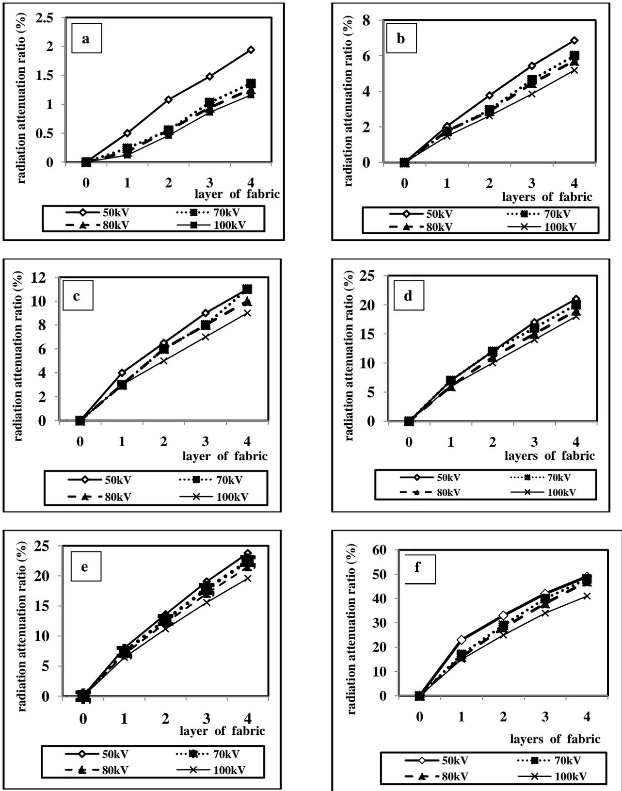
**Figure 6.** Radiation attenuation ratios of the uncoated (a) and coated fabrics (1-4 layers) with barium sulphate at different concentration (b-f): (b) 10% (w/w); (c) 20% (w/w); (d) 30% (w/w); (e) 40% (w/w) and (f) 50% (w/w).
