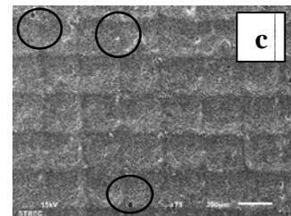
**Figure 5.** SEM micrographs of coated fabrics with barium sulphate at different concentration of 50% (w/w) after rubbing and washing tested: (a) after rubbing tested in dry condition; (b) after rubbing tested in wet condition and (c) after washing tested.
