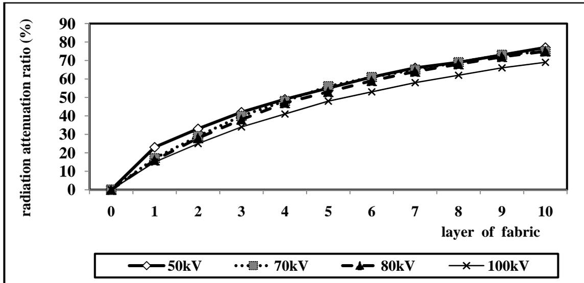
**Figure 7.** Radiation attenuation ratios of the coated fabrics at 1-10 layers with barium sulphate at concentration of 50% (w/w).
