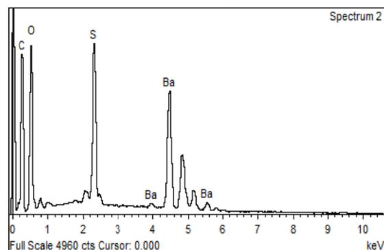
**Figure 3.** EDS spectra of the coated fabrics with barium sulphate at concentration of 50% (w/w).
