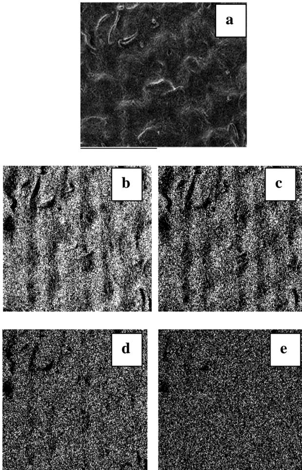
**Figure 4.** Mapping of elements on the cotton fabric coated with the barium sulphate at concentration of 50%(w/w): (a) SEM micrograph of the coated fabric; (b) mapping of C element; (c) mapping of O element; (d) mapping of S element and (e) mapping of Ba element.
