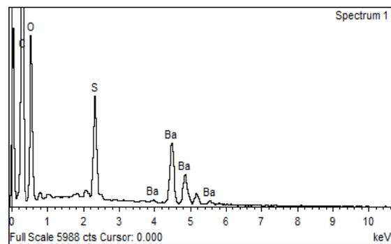
**Figure 2.** EDS spectra of the coated fabrics with barium sulphate at concentration of 10% (w/w).
