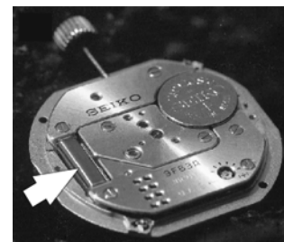
Figure 1. Use of the superfine wires in the fields of precision equipment and semiconductor: magnet wire for wristwatch (courtesy of SEIKO Corp.).
