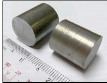
Figure 3. Geometry of AISI 1015 and AISI 4115 samples for the study, i.e. quenching, hardness test and microstructural examination.
