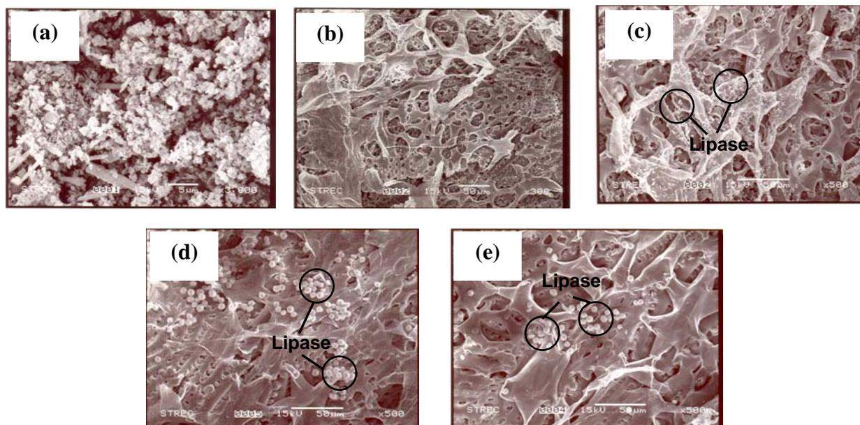
**Figure 3.** SEM images of free lipase (a); ground *Cyperus papyrus* L. fiber (b); immobilized lipase by physical adsorption in heptane, Im-ADHEP (c); immobilized lipase by physical adsorption in phosphate buffer solution, Im-ADPB (d); and by covalent binding, Im-CB (e) onto ground *Cyperus papyrus* L.
