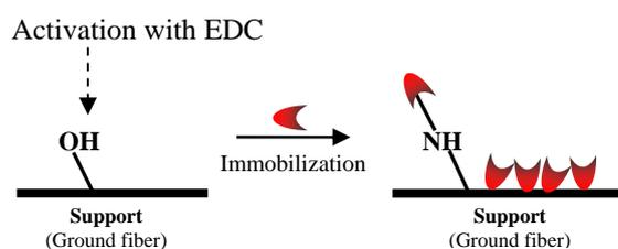
**Figure 1.** Schematic illustration of lipase immobilization techniques.
