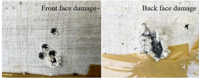
Figure 9. Depicts front and back face damage post projectile impact.
