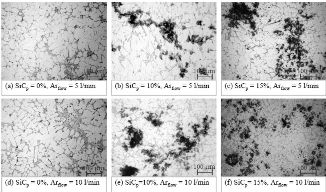
**Figure 2.** Microstructures at 620 °C casting temperature
