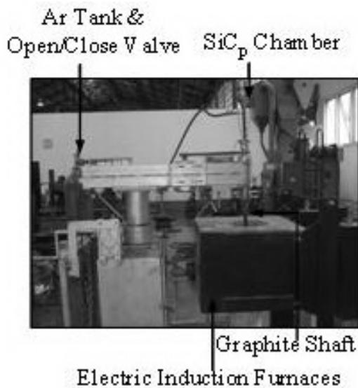
**Figure 1.** The modified  $\text{SiC}_p$  Injection Mobile Degassing Unit ( $\text{SiC}_p$ -IMDU)
