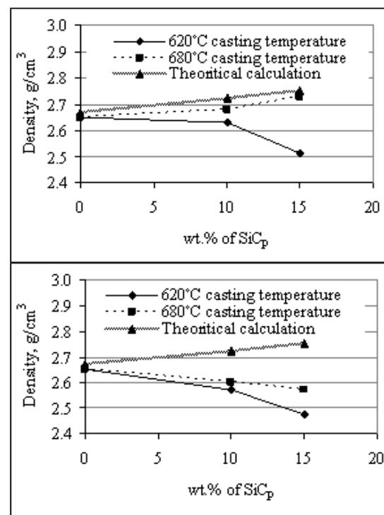
**Figure 4.** Density of  $\text{SiC}_p$ -Al composite
