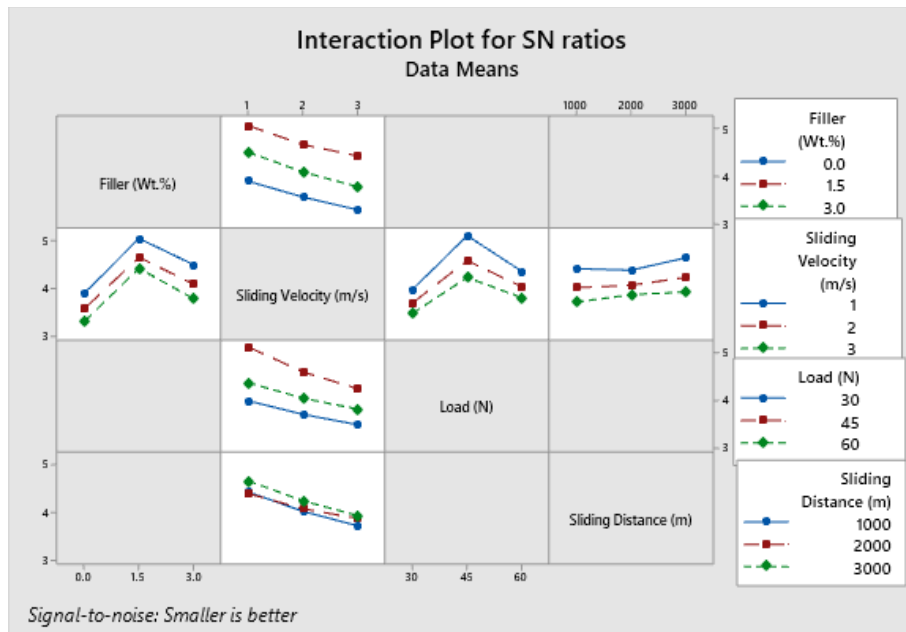
Figure 7. Interaction plots of SNR for Ks for mono and HAP filled hybrid CF/Ep composites.
