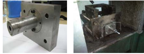
Figure 3. The extrusion die and laboratory-scale machine used in this study.
