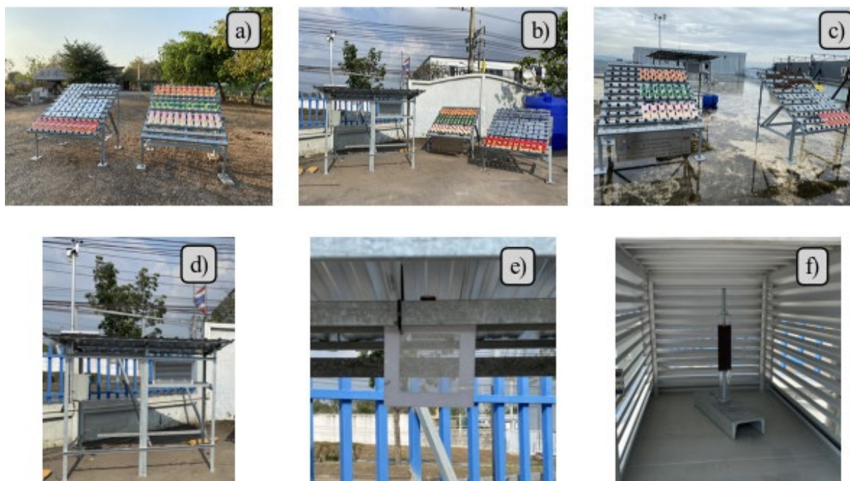
Figure 1. the test setup at Saraburi a), Chonburi b), and Songkhla c) together with the weather station d), dry gauze e) and lead cylinder f).
