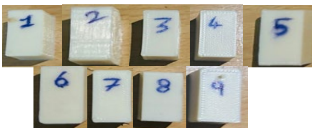
Figure 4. Compressive test samples.
