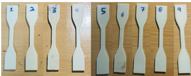
Figure 2. Tensile test samples.
