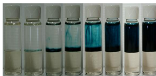
Figure 3. Polymerization through the \text{CHCl}_3 /water interface
