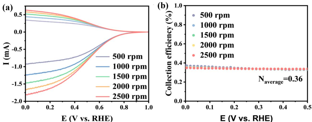
**Figure S6.** (a) RRDE voltammograms of glassy carbon electrode in 10 mM  $\text{K}_3\text{Fe}(\text{CN})_6$  and 0.1 M KCl with the disk and ring currents at 500, 1000, 1500, 2000 and 2500 rpm. The scan rate is  $5 \text{ mV}\cdot\text{s}^{-1}$  ( $1.3 \text{ V}$  vs. RHE for ring), (b) The corresponding collection efficiency of RRDE voltammograms as a function of the potential.
