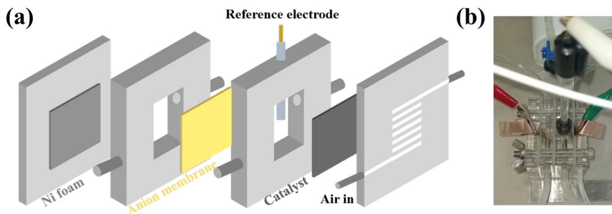
Figure S9. (a) The schematic diagram and (b) optical photograph of the flow cell.
