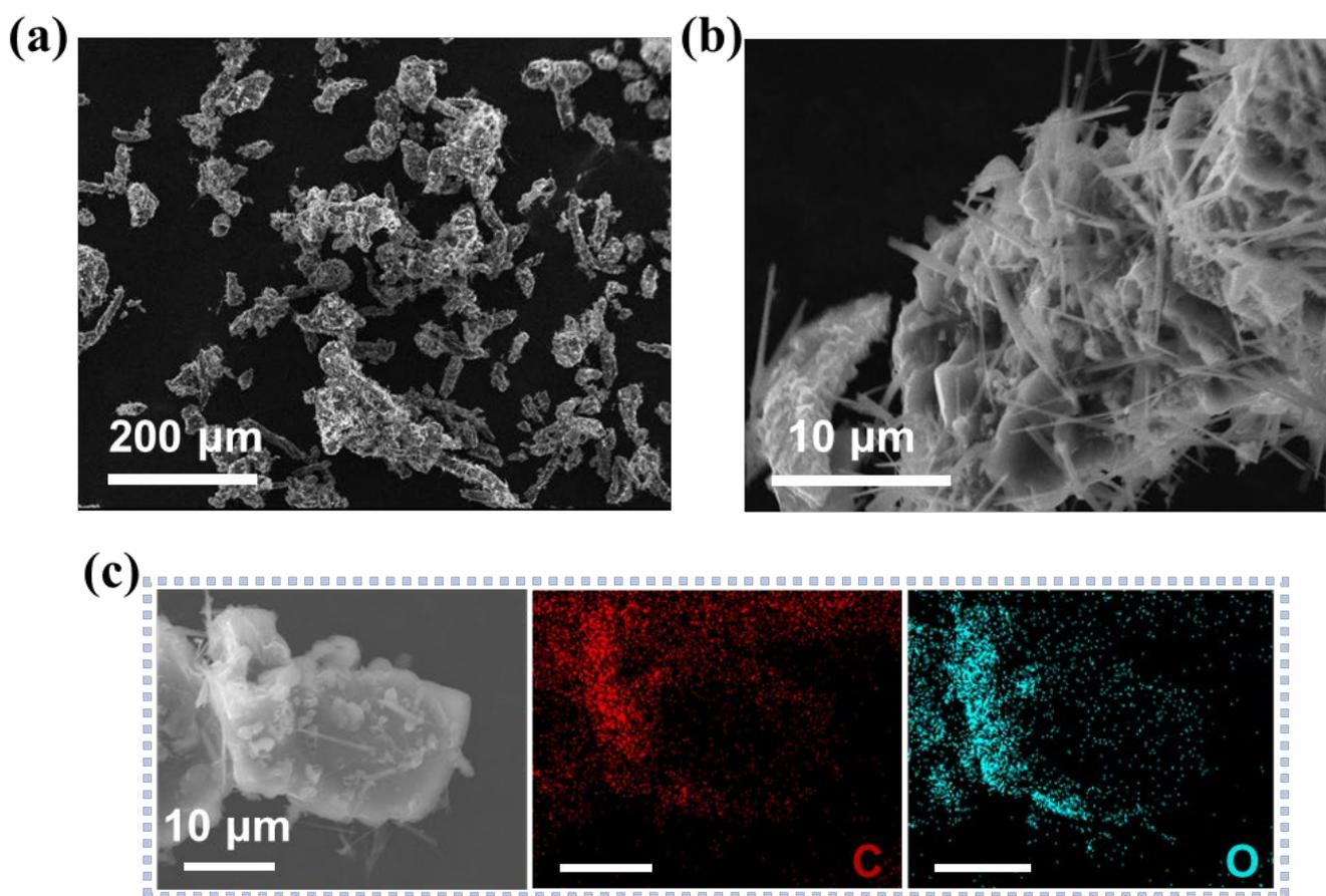
**Figure S1.** (a) and (b) SEM images, (c) EDS elemental mappings of HC.
