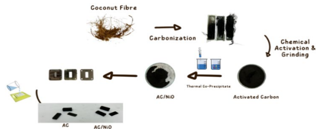
Figure 1. Schematic illustrations show the process from coconut fiber to composite material.
