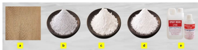
Figure 1. Photographic images of (a) Hemp fiber mat; (b) Al 2 O 3 NPs; (c) SiO 2 NPs; (d) MgO NPs and (e) Matrix materials.
