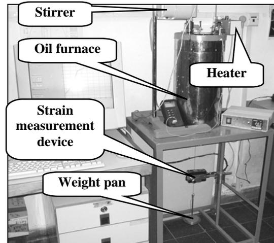
Figure 1. A view of the creep tester
