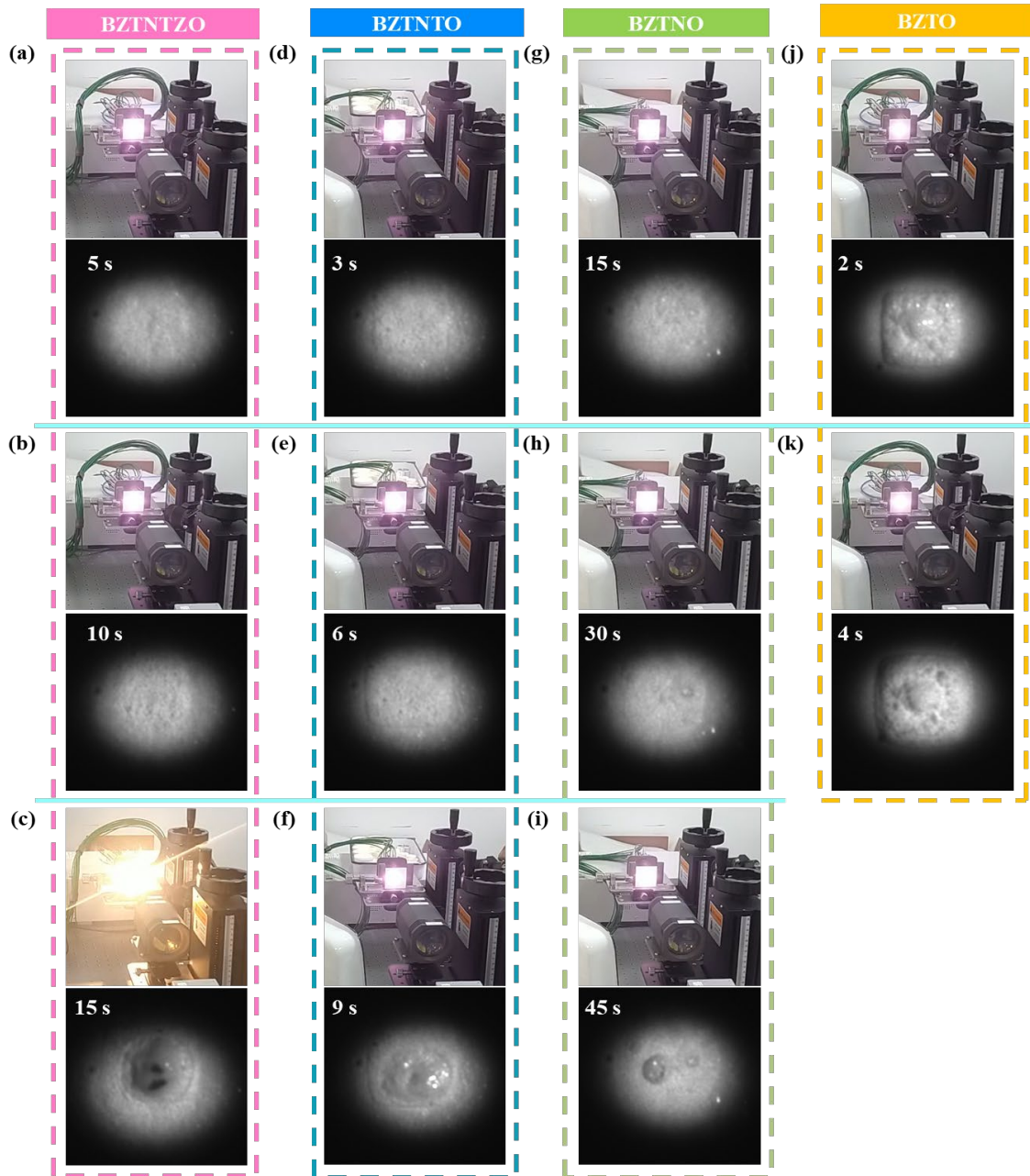
Figure 1. Irradiation status (top) and in-situ molten pools (below) of (a-c) BZTNTZO, (d-f) BZTNTNO, and (g-i) BZTNO at 1500 W·cm -2 , and (j-k) BZTO at 1000 W·cm -2 during fixed time intervals.
