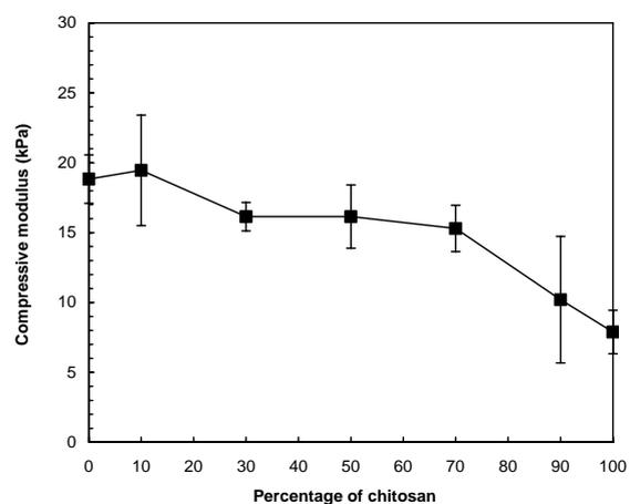
**Figure 2.** Compressive modulus of collagen/chitosan scaffolds with different blending composition
