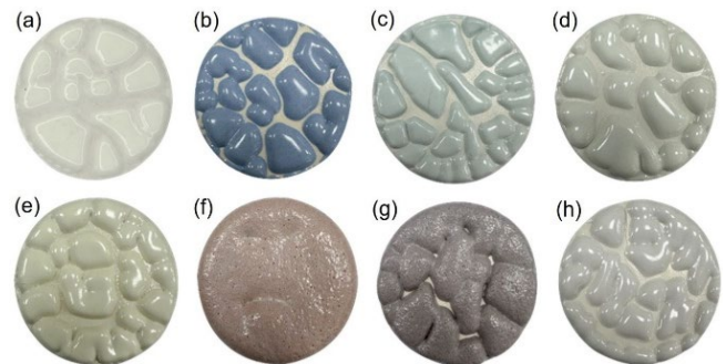
Figure 14. The glaze samples (10 wt% MgO) with addition of ceramic stains in the amount of 5 wt%. (a) Unadded, (b) Purple, (c) Blue, (d) Green, (e) Yellow, (f) Orange and (g) Red. All stains were from Amarin Ceramics.
