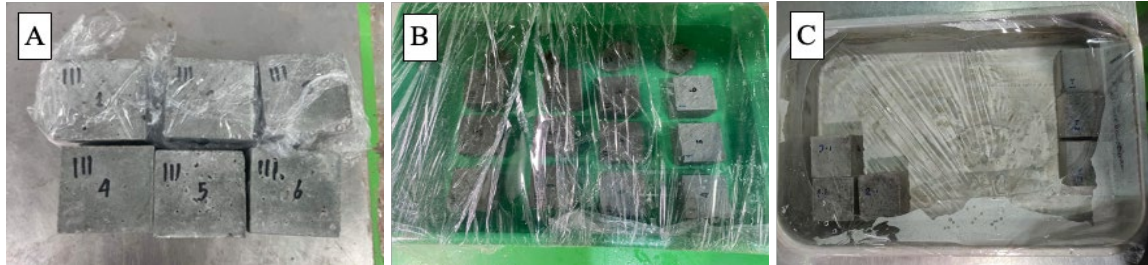
Figure 1. Samples under two testing conditions: (a) ambient temperature, (b) sodium chloride solution, and (c) magnesium sulfate solution.
