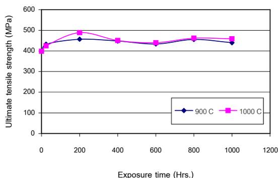
**Figure. 11** The relationship between ultimate tensile strength and aging time
