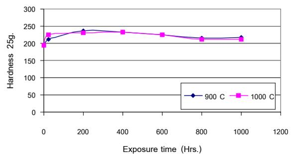
**Figure. 9** The relationship between micro hardness tests (HV25g) of matrix and exposure time
