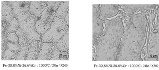
**Figure. 4** Microstructure of specimen after aging at 1000°C for 24 hours; Low magnification (Left) and High magnification (Right)
