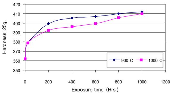
**Figure. 10** The relationship between micro hardness Tests (HV 25g) of primary carbide and exposure time
