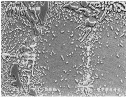
**Figure. 5** SEM micrograph of specimen after aging at 900°C for 24 hours
