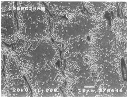
**Figure. 6** SEM micrograph of specimen after aging at 1000°C for 24 hours
