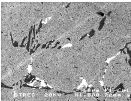
**Figure. 7** SEM micrograph of specimen after aging at 900°C for 1000 hours
