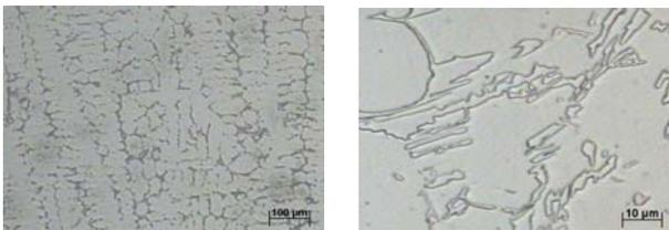
**Figure. 1** Microstructure of as-received material; Low magnification (Left) and High magnification (Right)
