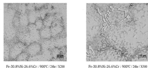
**Figure. 3** Microstructure of specimen after aging at 900°C for 24 hours; Low magnification (Left) and High magnification (Right)
