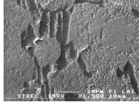
**Figure. 8** SEM micrograph of specimen after aging at 1000°C for 1000 hours
