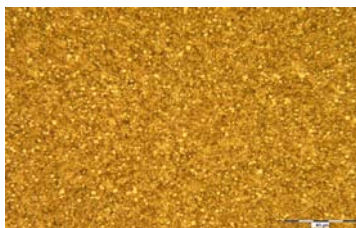
Figure 1. The structure of high-speed steel Vanadis 4, etched.
