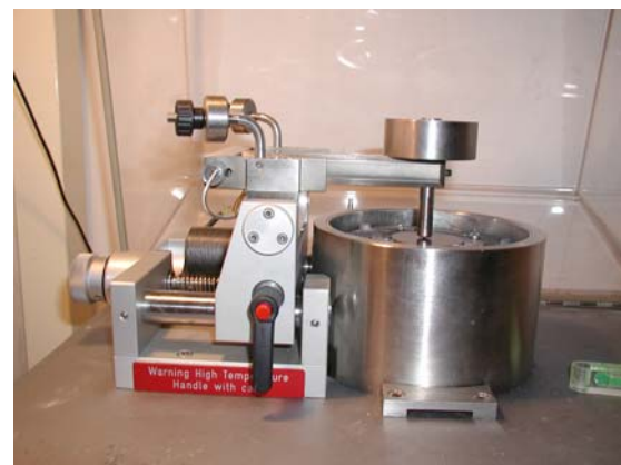
Figure 16. CSM High temperature tribometer
