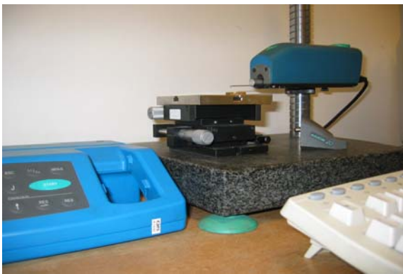
Figure 11. Profilometer Hommel Tester T 1000
