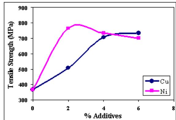
Figure 2. Ultimate tensile strength of 409L.
