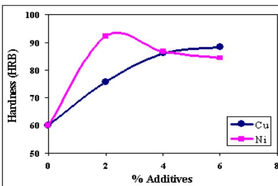
**Figure 5.** Hardness of 409L.
