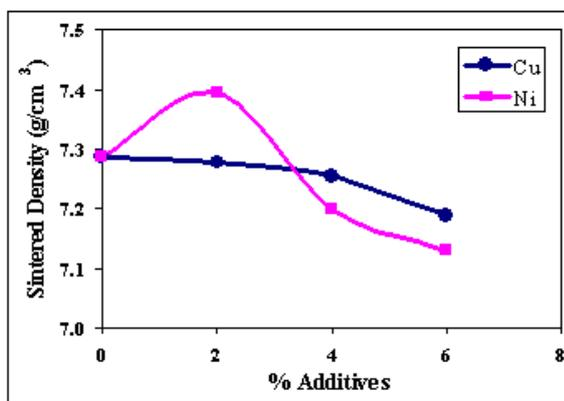
Figure 1. Sintered density of 409L.
